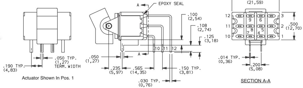
**AV3** VERTICAL RIGHT ANGLE, SNAP-IN, PC THRU-HOLE,
