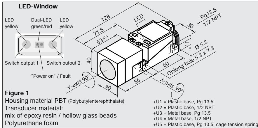
The measurement of distance is derived from the propagation time of the ultrasonic pulse. Thus, the microprocessor is able to calculate the range as a function of the propagation time and the velocity of sound.
