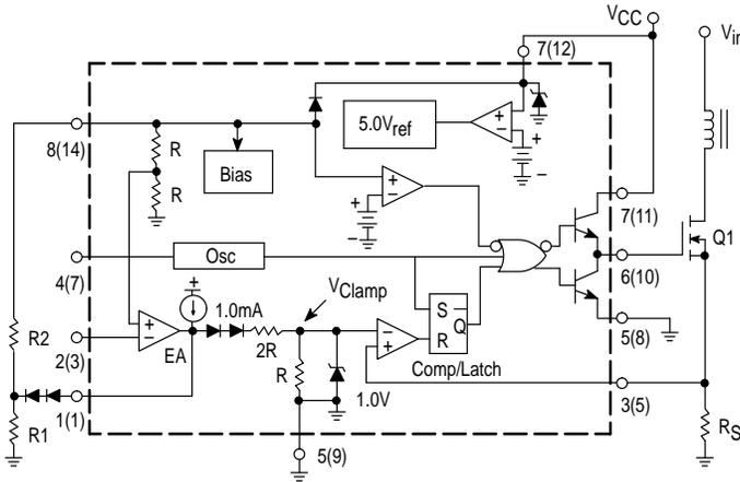
$$V_{Clamp} = \frac{1.67}{\left(\frac{R_2}{R_1} + 1\right)} + 0.33 \times 10 - 3 \left(\frac{R_1 R_2}{R_1 + R_2}\right) \quad I_{pk(max)} = \frac{V_{Clamp}}{R_S}$$
