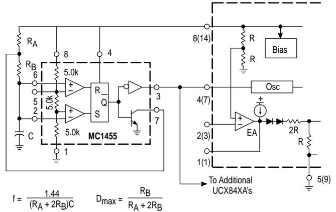
$$f = \frac{1.44}{(R_A + 2R_B)C} \quad D_{max} = \frac{R_B}{R_A + 2R_B}$$
