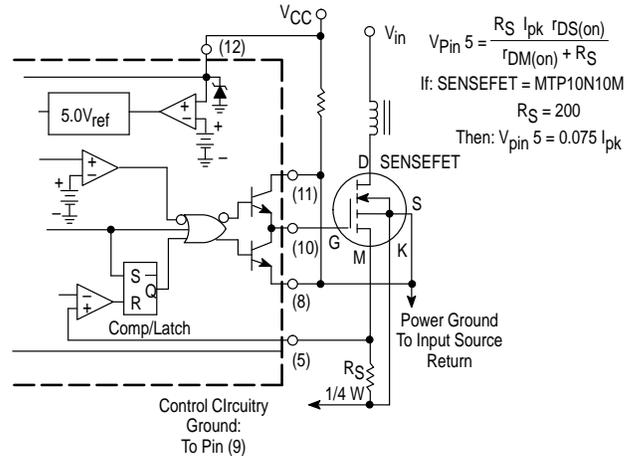
$$V_{pin 5} = \frac{R_S I_{pk} r_{DS(on)}}{r_{DM(on)} + R_S}$$
