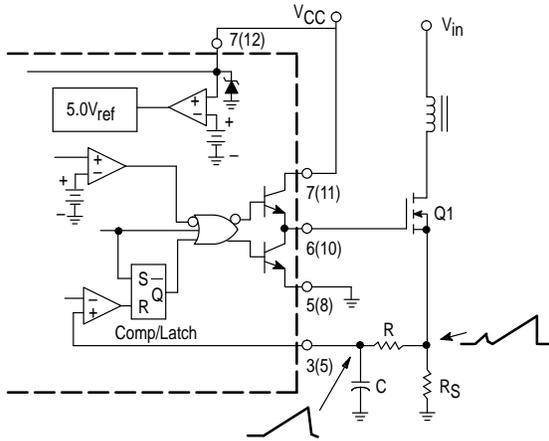
The addition of the RC filter will eliminate instability caused by the leading edge spike on the current waveform.
