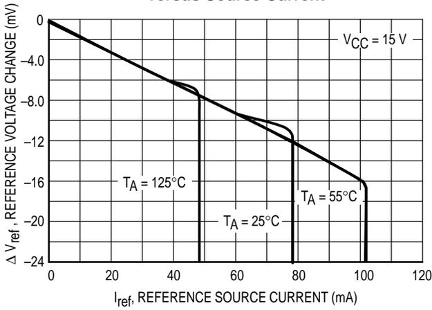
Figure 10. Reference Short Circuit Current versus Temperature
