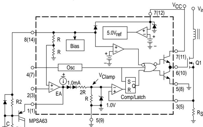
$$V_{Clamp} = \frac{1.67}{\left(\frac{R_2}{R_1} + 1\right)} \quad I_{pk(max)} = \frac{V_{Clamp}}{R_S} \quad \text{Where: } 0 \leq V_{Clamp} \leq 1.0 \text{ V}$$
