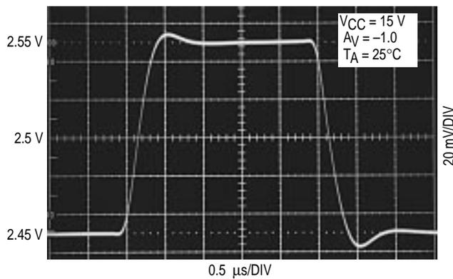
Figure 6. Error Amp Large Signal Transient Response
