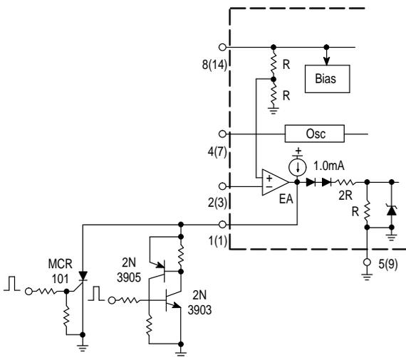
The MCR101 SCR must be selected for a holding of less than 0.5 mA at  $T_A(\text{min})$ . The simple two transistor circuit can be used in place of the SCR as shown. All resistors are 10 k.
