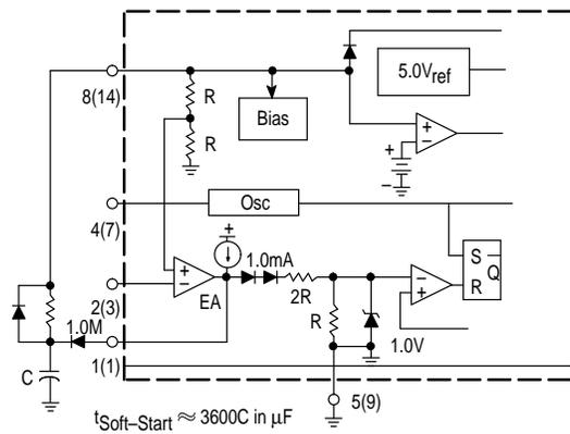
$$t_{Soft-Start} \approx 3600C \text{ in } \mu\text{F}$$
