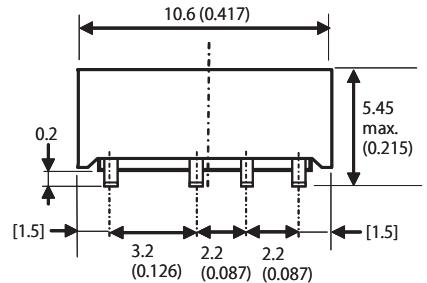
Tolerance of lead pitch is  $\pm 0.15\text{mm}$  (0.006inch)
