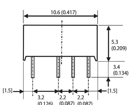
Tolerance of lead pitch is  $\pm 0.15\text{mm}$  (0.006inch)
