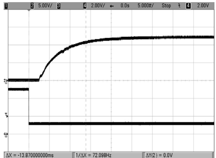
Enable Start-up (Vin=48V, Iout=5A, Cload=1000μF Ta=+25°C) Trace 2=Output, Trace 4= Enable.
