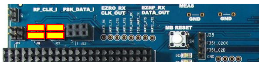
Figure 16. Radio Power Headers Diagram (EBID Powered by 3.3 V)
