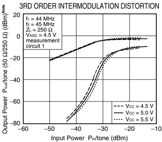
**Note** Measurement value with spectrum analyzer.
