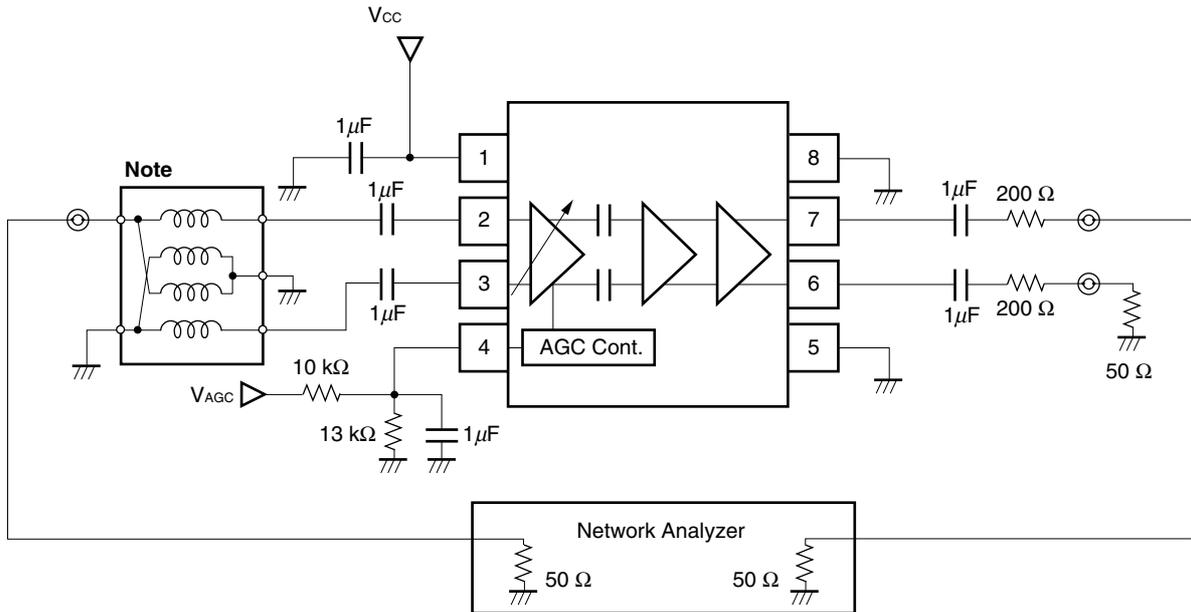
**Note** Balun Transformer: TOKO 617DB-1010 B4F (Double balanced type)
