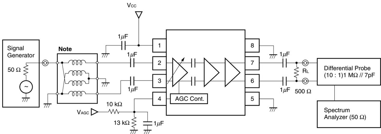
**Note** Balun Transformer: TOKO 617DB-1010 B4F (Double balanced type)
