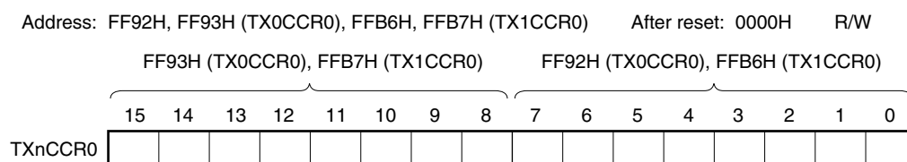
Figure 6-4. Format of 16-bit timer Xn capture/compare register 0 (TXnCCR0)
