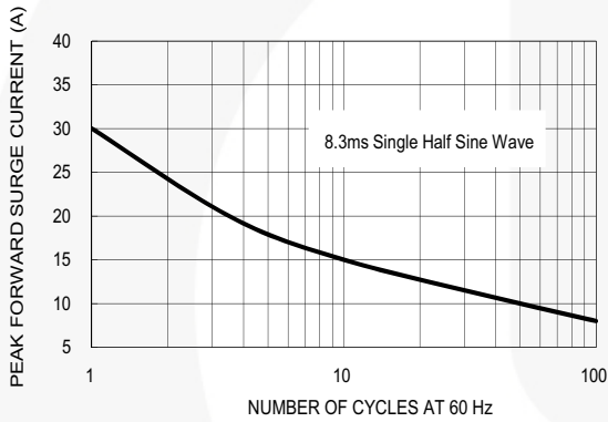
Figure 3. Maximum Non-Repetitive Forward Surge Current
