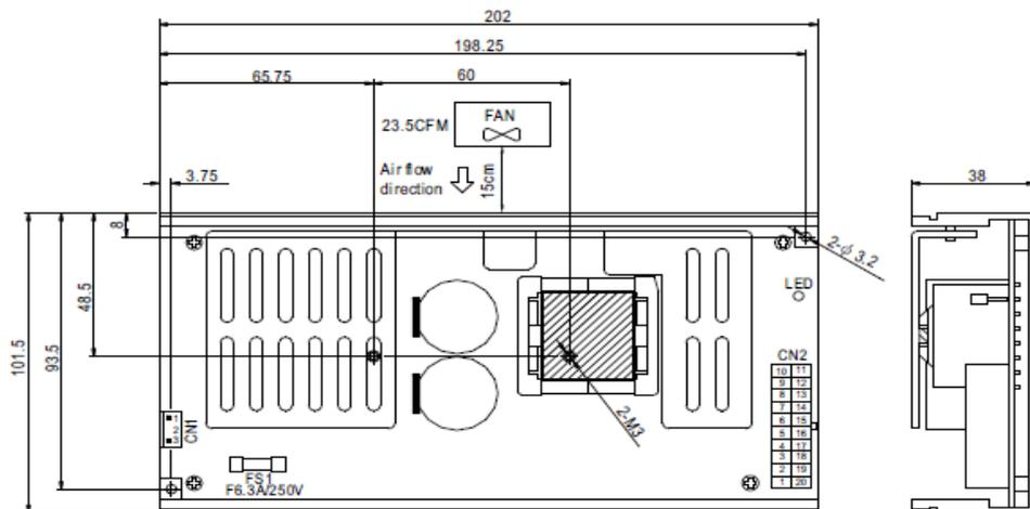
AC Input Connector (CN1) : JST B3P-VH or equivalent
