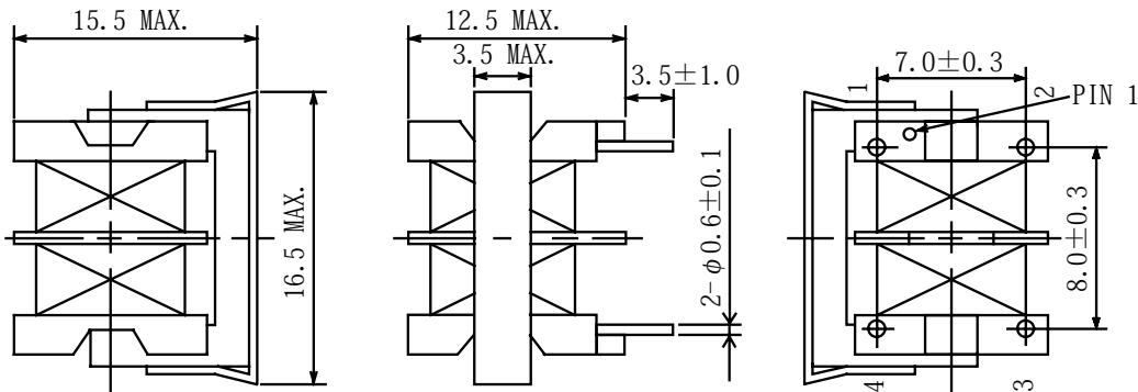
\* DIMENSION DOES NOT INCLUDE SOLDER USED ON COIL.
