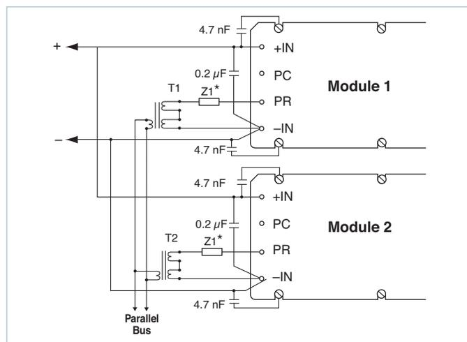
Figure 10 — Transformer-coupled interface
