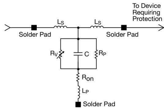
Where:  $R_v$  = Voltage Variable resistance (per VI curve)
