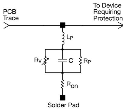
Where:  $R_v$  = Voltage Variable resistance (per VI curve)
