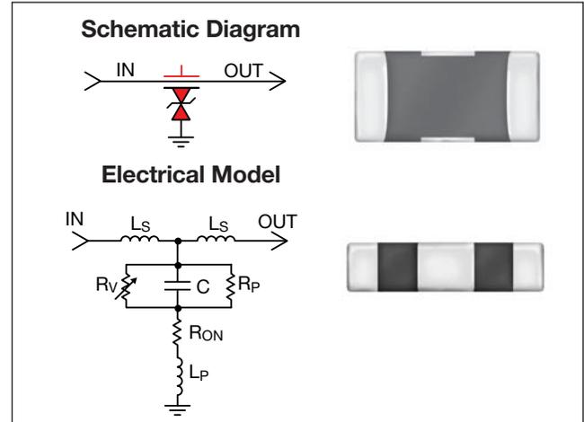
the TransFeed product. Not only is there significantly greater attenuation at a higher self-resonance frequency, but the roll-off characteristic becomes much flatter, resulting in EMI filtering over a much broader frequency spectrum. Typical applications include filtering/protection on Microcontroller I/O Lines, Interface I/O Lines, Power Line Conditioning and Power Regulation.
