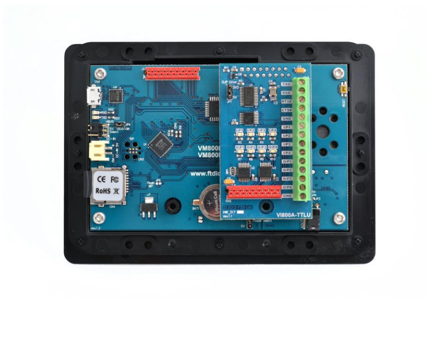
Figure 5-1 - VI800A-TTLU module connected to VM800P Plus module
