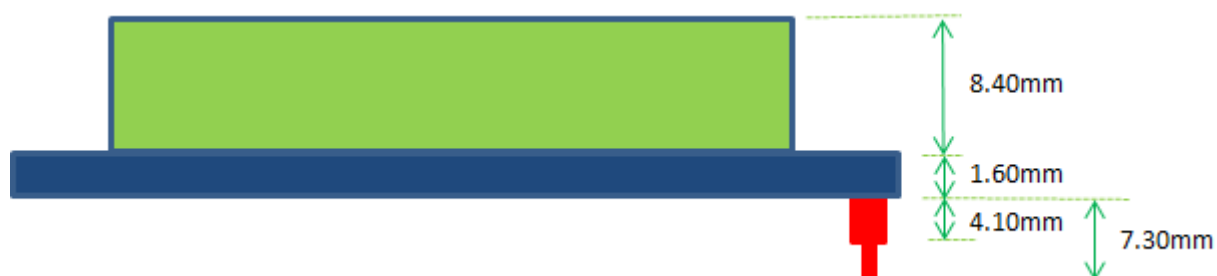
Figure 3-4 - VI800A-TTLU module PCB Side view
