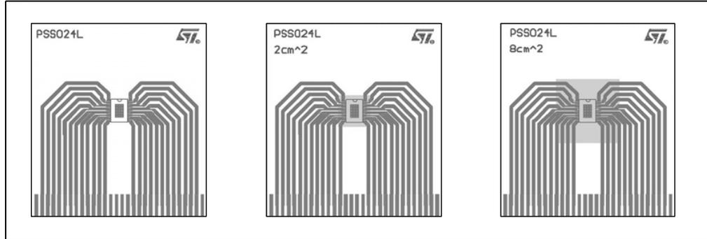
Note: Layout condition of  $R_{th}$  and  $Z_{th}$  measurements (PCB: Double layer, Thermal Vias, FR4 area= 77 mm x 86 mm, PCB thickness=1.6mm, Cu thickness=70  $\mu$ m (front and back side), Copper areas: from minimum pad lay-out to 8 cm<sup>2</sup>).
