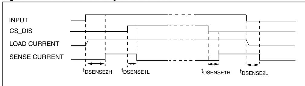
**Figure 5. Delay response time between rising edge of output current and rising edge of current sense (CS enabled)**
