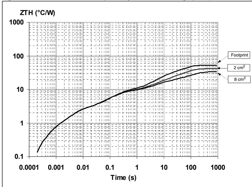
Figure 31. Thermal fitting model of a double channel HSD in PowerSSO-24<sup>(a)</sup>
