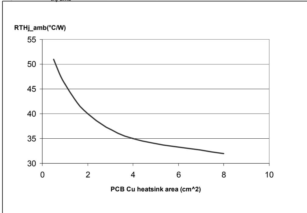
Figure 30. PowerSSO-24 thermal impedance junction ambient single pulse (one channel on)
