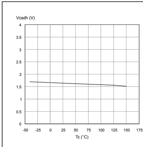
Figure 23. CS\_DIS clamp voltage
