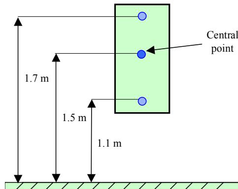
The field strength value to be used in further calculations is the averaged value of the three values, obtained for each spatial point :
