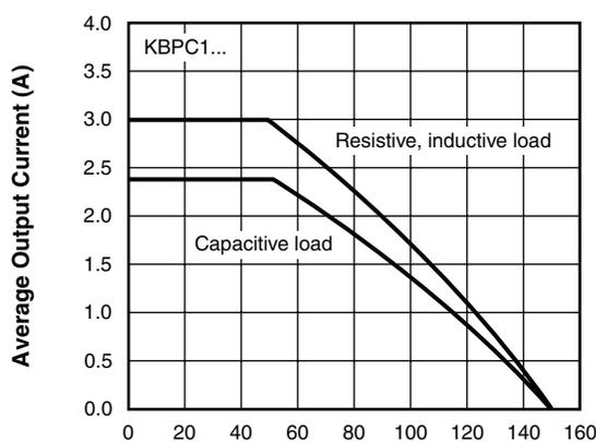
93585\_01 Maximum Allowable Case Temperature ( $^\circ\text{C}$ )
