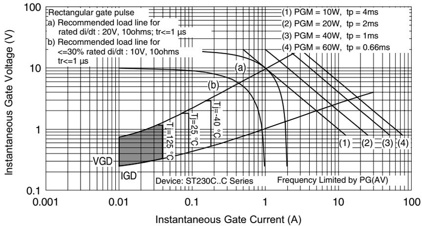
Fig. 11 - Gate Characteristics
