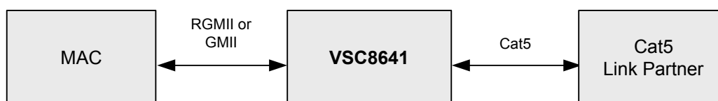
Figure 3. RGMII or GMII to Cat5 Block Diagram
