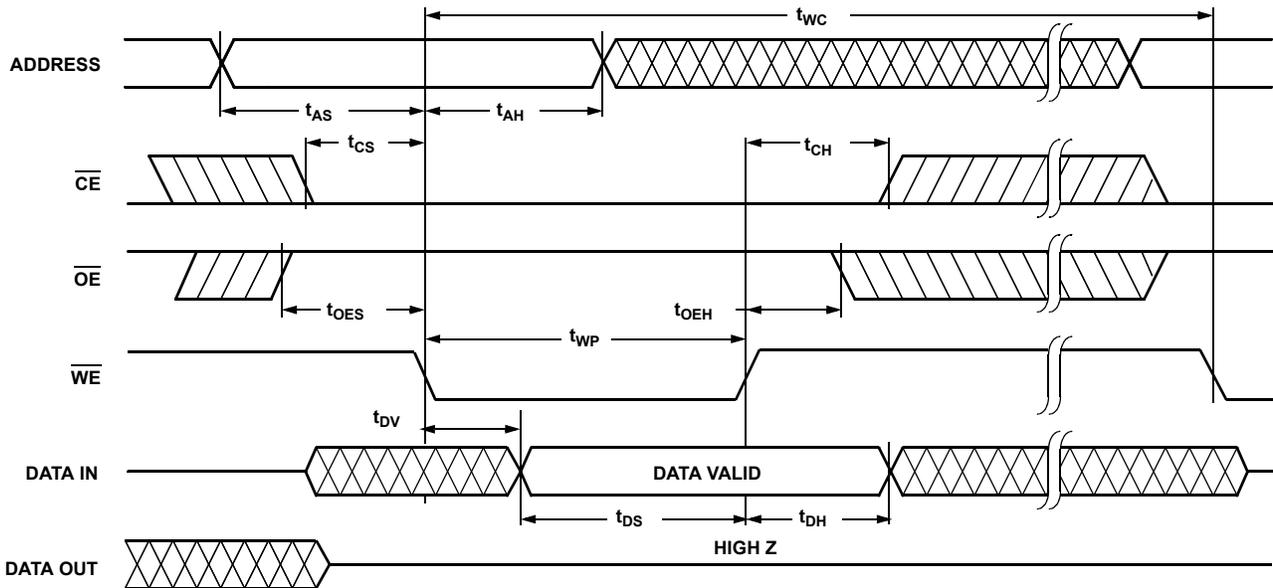
**$\overline{CE}$  Controlled Write Cycle**
