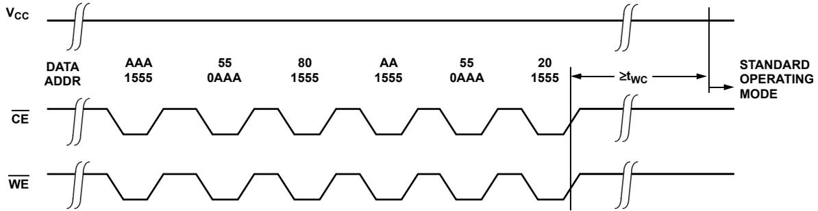
**FIGURE 8. RESET SOFTWARE DATA PROTECTION TIMING SEQUENCE**
