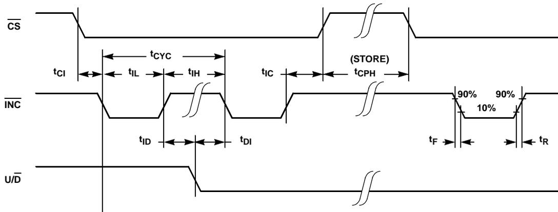
Note:  $\overline{CS}$ ,  $\overline{INC}$ ,  $U/\overline{D}$ ,  $R_H$  and  $R_L$  are used to refer to either  $\overline{CS}_1$  or  $\overline{CS}_2$ , etc.
