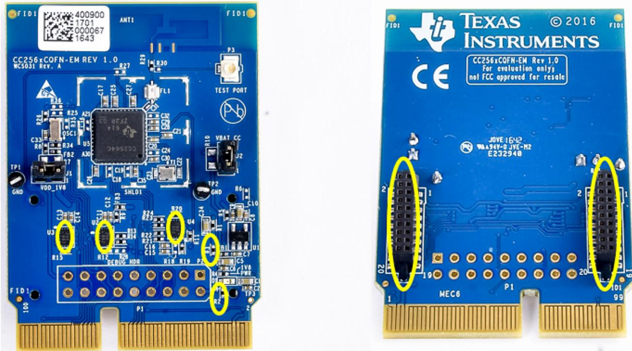
**Figure 6. CC256XCQFN-EM Hardware Modifications for COM Connector**
