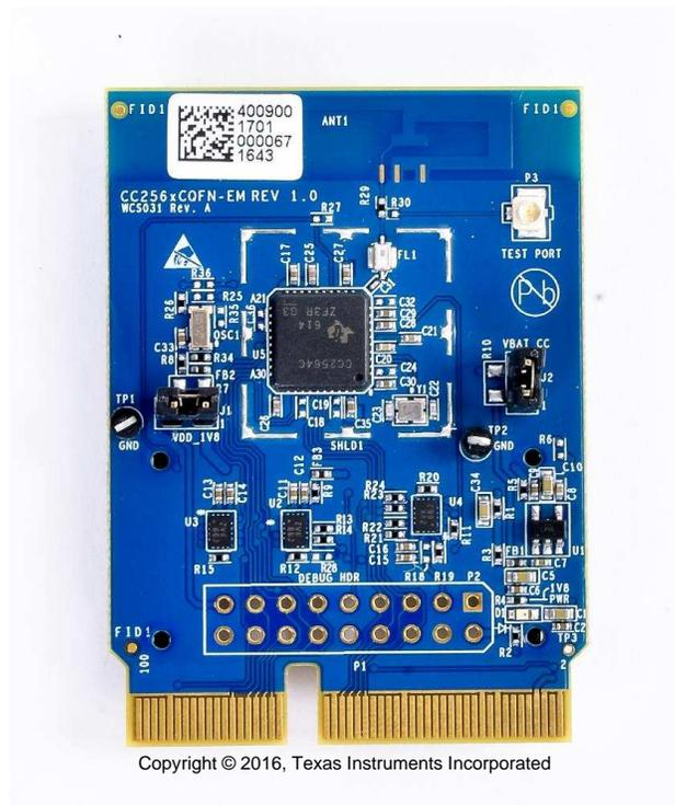
**Figure 1. CC256xCQFN-EM Board**
