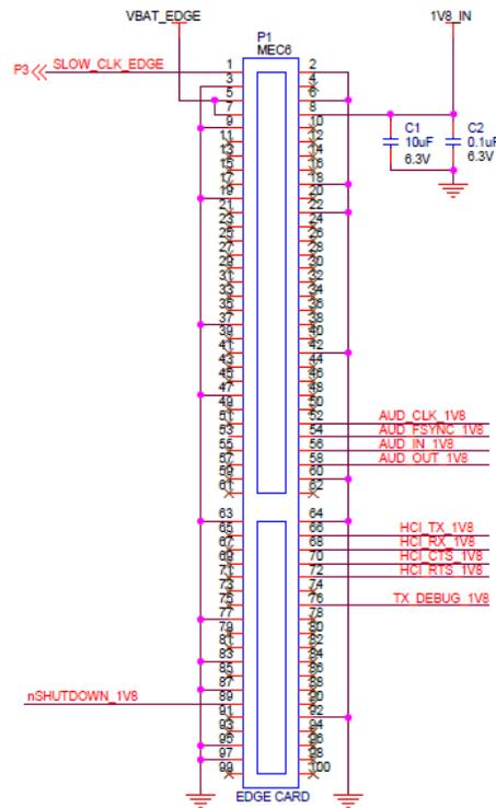
**Figure 5. COM Connector Pinout**
