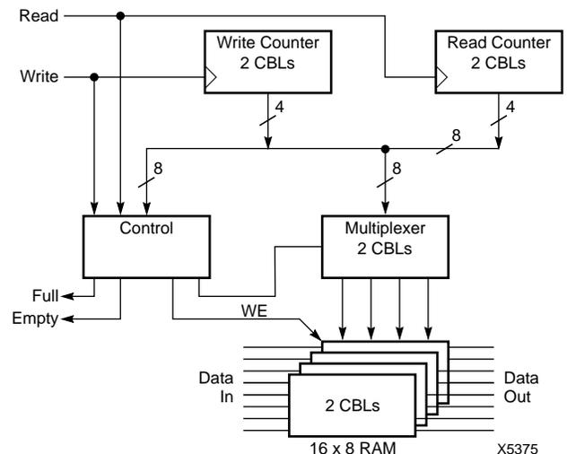
Figure 4. 16-byte FIFO
