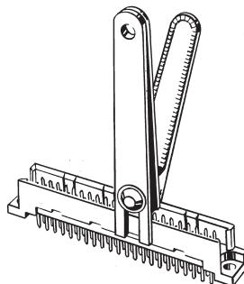
Cut the Coding Key on the Plug and insert the Coding Key in the Coding Key slots on the Socket to prevent improper insertion of the Plug into the Socket.
