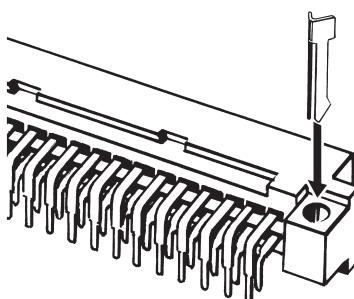
Fastening pins (XC5Z-0002) are used to keep the connector flush against the board during automated soldering.
