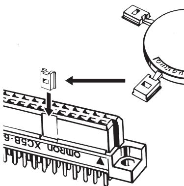
2. Insert the special Coding Key (XC5Z-0001) into the Coding Key slots in the housing wall of the corresponding Socket.
