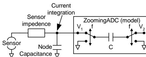
**Figure 20 - The Switched Capacitor Principle**
