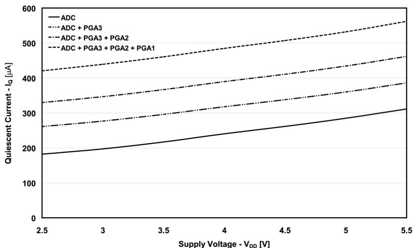
**Figure 29 - Quiescent Current Consumption vs. Supply Voltage**
