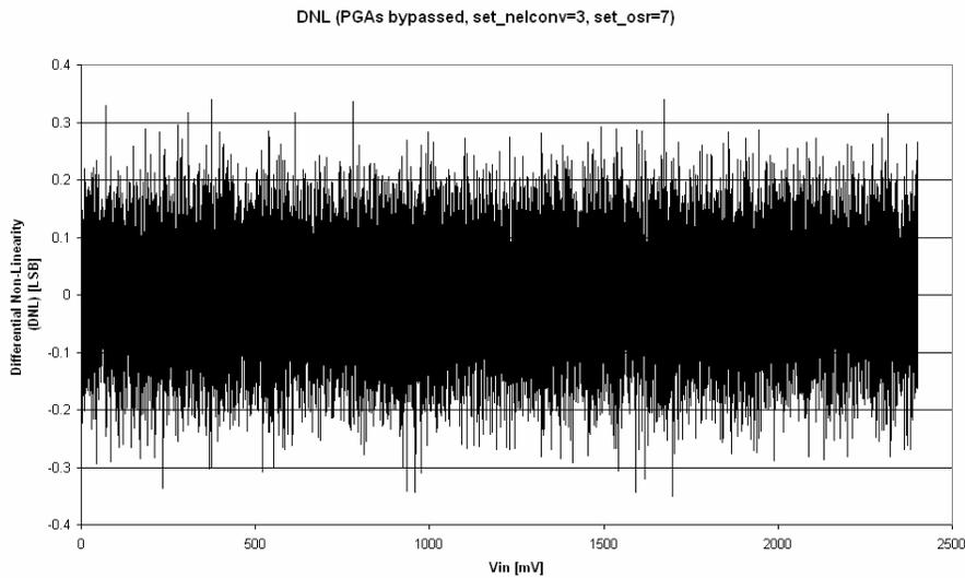
**Figure 23 - Differential Non-Linearity of the ADC Converter**
