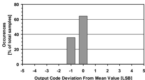
Figure 24 - ADC Noise (PGA1, 2 & 3 Bypassed, OSR = 512,  $N_{ELCONV} = 2$ )
