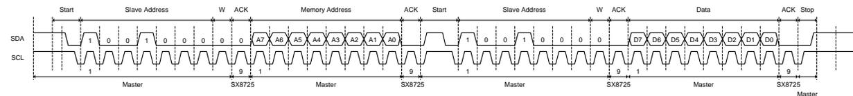
**Figure 6 - Timing Diagram for Writing to the SX8725**
