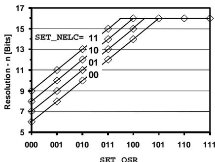
**Figure 12 - Resolution vs. SET\_OSR[2:0] and SET\_NELC[1:0]**
