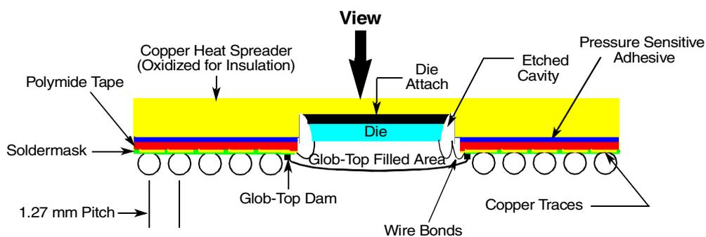
Figure 14. Side View of the TBGA Package
