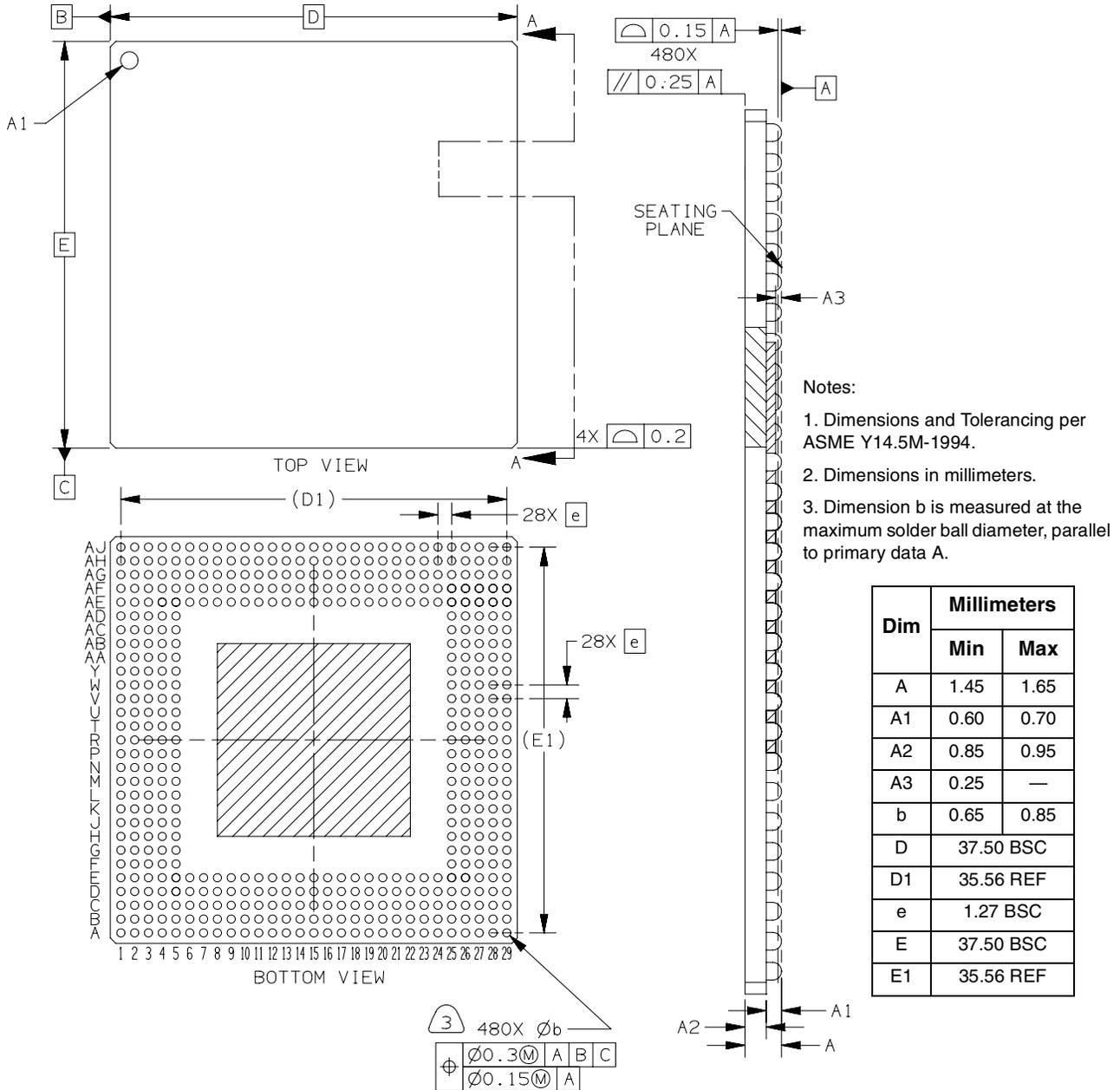
Figure 15. Mechanical Dimensions and Bottom Surface Nomenclature
