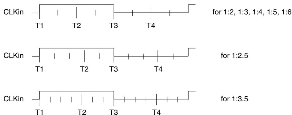
Figure 12. Internal Tick Spacing for Memory Controller Signals
