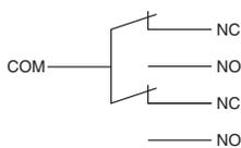
Note: The NO and NC terminal arrangement is reversed for Models with reverse operation (Z-10FM).
