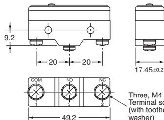
**Note:** With reverse action models (Z-15GM), the positions of NO and NC terminals are reversed.
