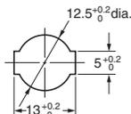
**Note:** Mount using either the side mounting holes or the panel mount plunger, not both. If using the side mounting holes, then remove the hexagonal nut(s) from the panel mount plunger.
