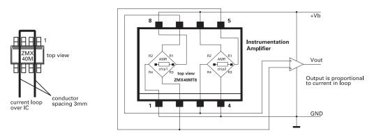
This double chip solution with the current loop conductor guarantees good rejection of external fields and a high isolation voltage.
