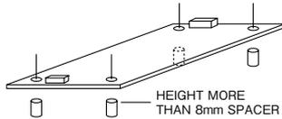
And allowable area by metal pieces is 9mm from each PCB corners. Refer to figure below.
