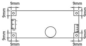
Please leave 4mm space from the surfaces and the sides of PCB, especially from the solder surface, 8mm space is necessary. If the space is not enough, the specification of insulation and withstand will not be satisfied.
