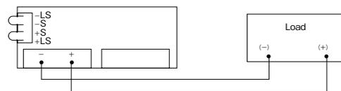
(2) When using remote sensing
