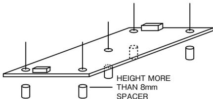
Please left 5mm space from the surfaces and left 4mm space from the sides of PCB, especially from the solder surface, 8mm space is necessary.
