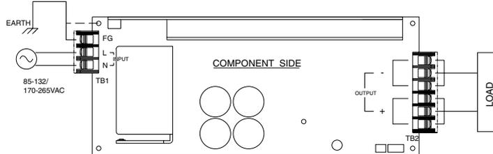
● The output current on one terminal is limited to 30A
