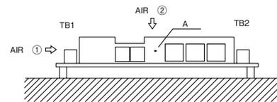
Please make air flow to maintain the heat sink (part A) temperature 85°C or less. (Operating ambient temperature is 50°C).
