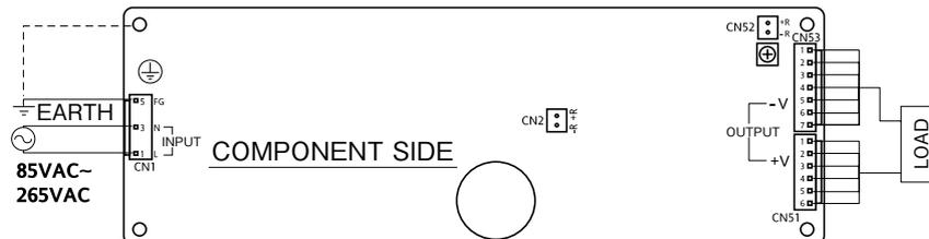
\* Connector for Remote ON/OFF Control : CN2, CN52 (J.S.T)
