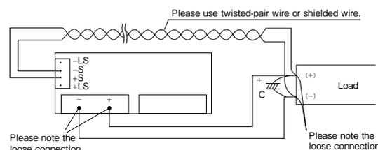
■ When the function of remote sensing is not used, connect +S terminal to +LS terminal, -S terminal to -LS terminal by short piece.
