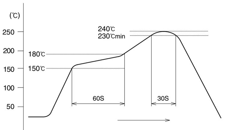
The temperature profile is based on the left conditions.
