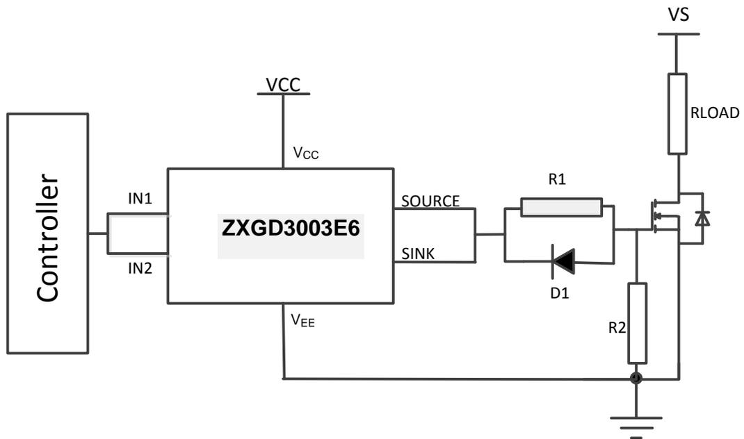
R1, D1 combination can be used for variable turn on and turn off times.
