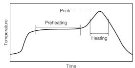
For soldering (Example: Sn/Pb)
