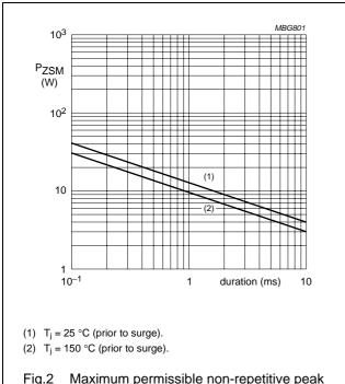
Fig.2 Maximum permissible non-repetitive peak reverse power dissipation versus duration.
