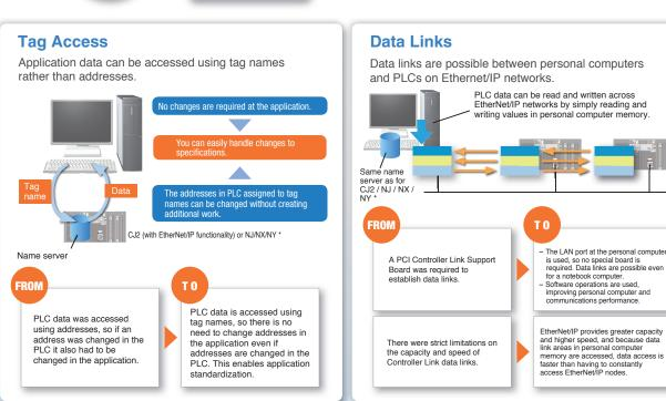
Note: The Network Configurator included in the CX-One Package or Sysmac Studio is required to set tag data links.
