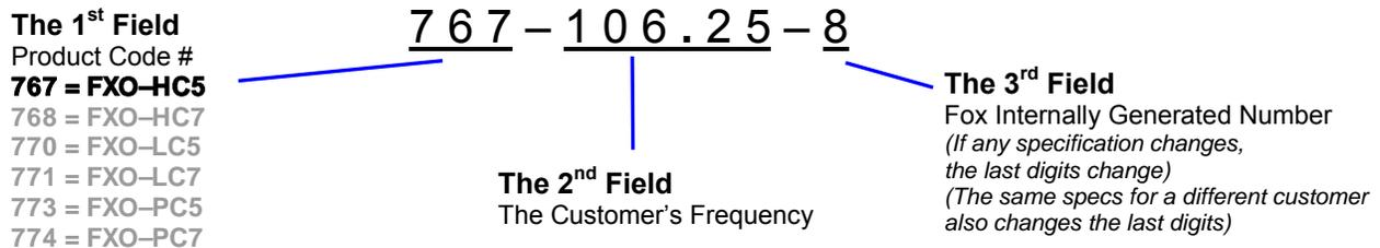
*This example, **FXO-HC536R-106.25** = HCMOS Output, Ceramic 5 x 3.2mm Package, 3.3V, ±25 PPM Stability, -40 to +85°C Temperature Range, at 106.25 MHz*
