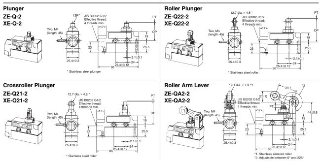
Note: 1. Unless otherwise specified, a tolerance of ±0.4 mm applies to all dimensions.
