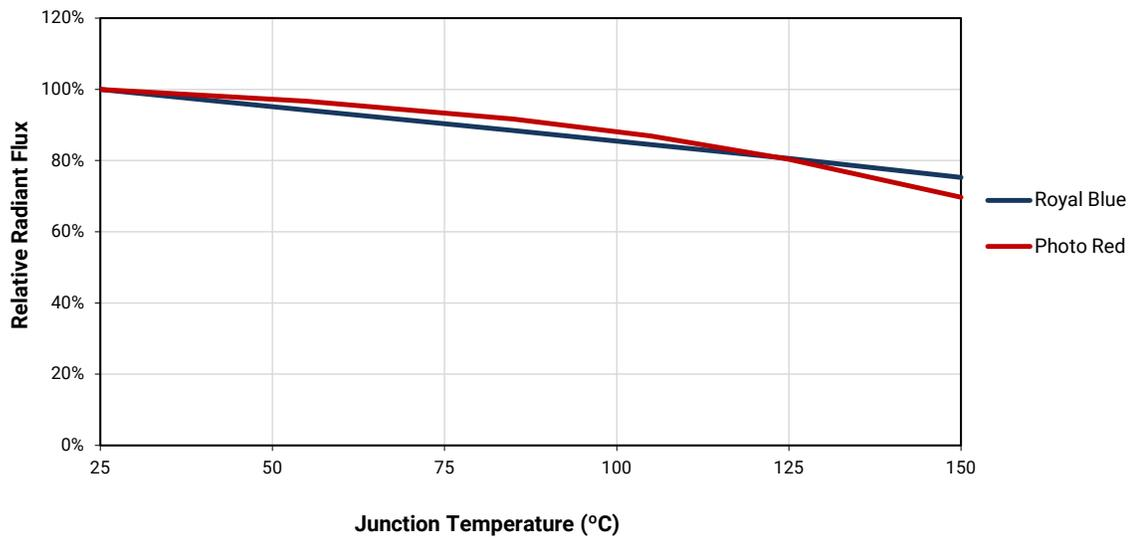
RELATIVE FLUX VS. JUNCTION TEMPERATURE ( $I_F = 350 \text{ mA}$ ) - CONTINUED
