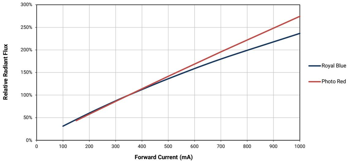
**RELATIVE FLUX VS. CURRENT ( $T_j = 25\text{ }^\circ\text{C}$ ) - CONTINUED**
