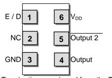
Terminations as viewed from the Top NOTE: XPRESSO LVPECL XOs are designed to fit on Industry Standard, 6 pad layouts
