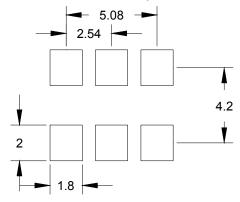
Note: XPRESSO LVPECL XOs are designed to fit on Industry standard, 6 pad, layouts.
