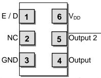
Terminations as viewed from the Top NOTE: XPRESSO LVPECL XOs are designed to fit on Industry Standard, 6 pad layouts
