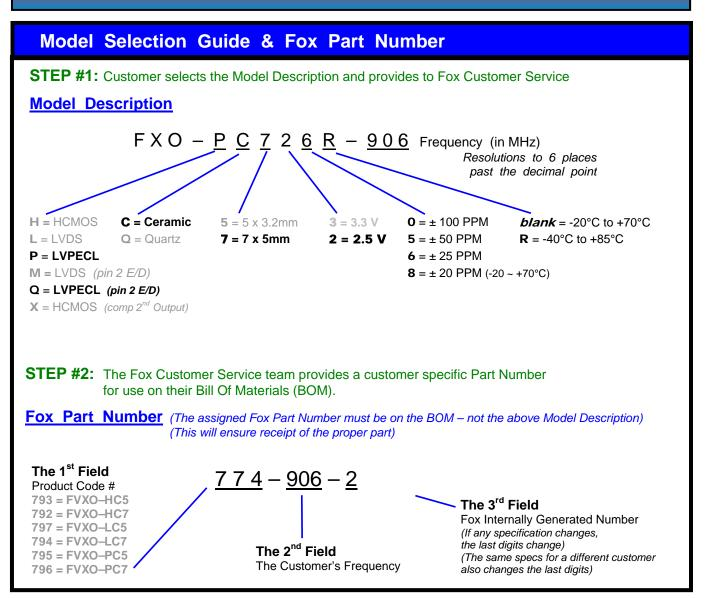
This example, FXO-PC726R-906 = LVPECL Output, Ceramic, 7 x 5mm Package, 2.5V, ±25 PPM Stability, -40 to +85°C Temperature Range, at 906 MHz
