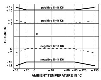
The temperature coefficient is guaranteed between  $-20 \,^{\circ}\text{C}$  to  $+85 \,^{\circ}\text{C}$ .
