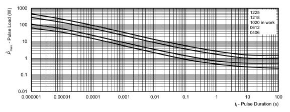
Maximum pulse load, single pulse; applicable if  $\bar{P} \to 0$  and n < 1000 and  $\hat{U} \le \hat{U}_{\text{max}}$ ; for permissible resistance change equivalent to 8000 h operation
