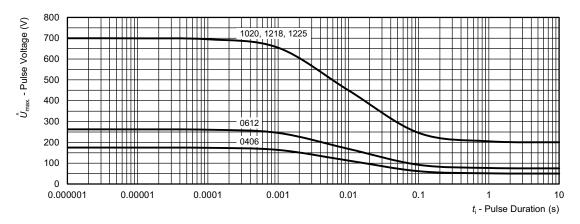
Maximum pulse voltage, single and continuous pulses; applicable if  $\hat{P} \leq \hat{P}_{\text{max}}$ ; for permissible resistance change equivalent to 8000 h operation
