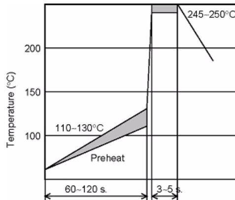
b. Soldering iron (recommended for Sn and Sn/Pb solders)
