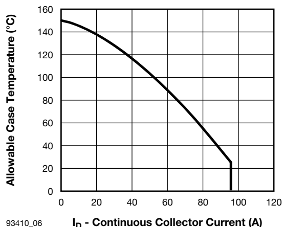
Fig. 6 - Maximum IGBT Continuous Collector Current vs. Case Temperature
