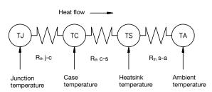
Thermal resistance:  $R_{th} j$ -c = junction to case
