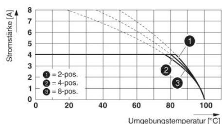
Derating curve for: PTPM 0.4/..-P-2.5 with PTSM 0.5/..-HH-2.5-THR R..
