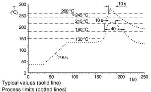
Vapour phase soldering
