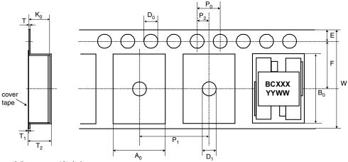
Cumulative pitch error: 0.2 mm over 10 pitches Cumulative tolerance over 10 holes: ± 0.2 mm
