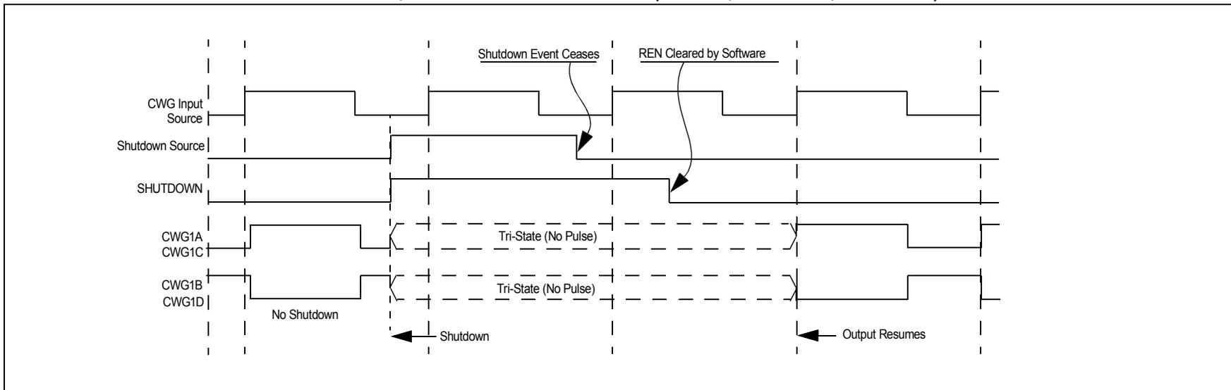
FIGURE 24-16: SHUTDOWN FUNCTIONALITY, AUTO-RESTART ENABLED (REN = 1, LSAC = 01, LSBD = 01)
