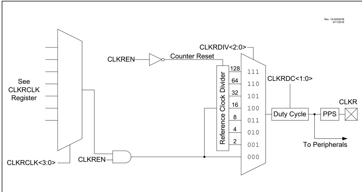
**FIGURE 5-2: CLOCK REFERENCE TIMING**
