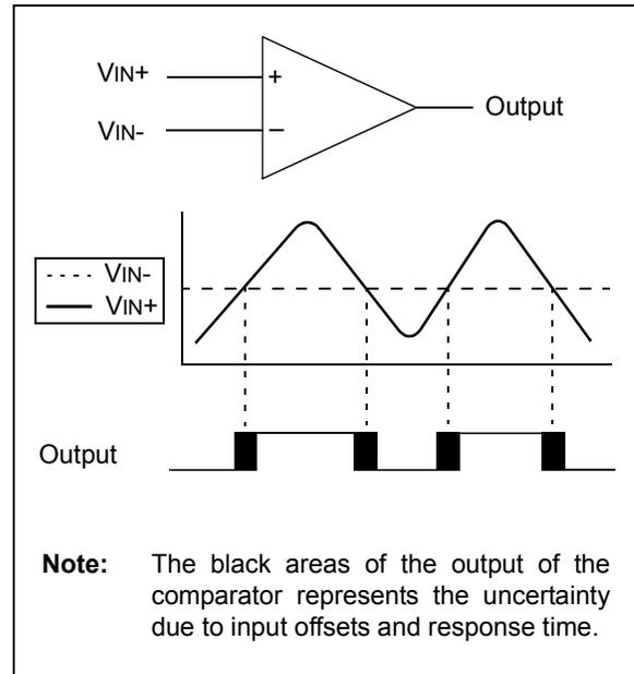
**FIGURE 32-2: COMPARATOR MODULE SIMPLIFIED BLOCK DIAGRAM**
