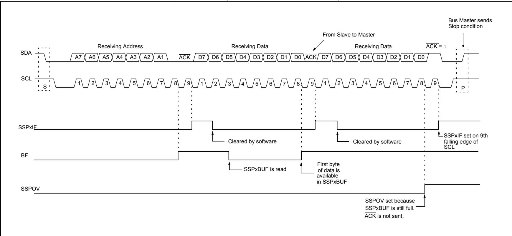
**FIGURE 26-15: I<sup>2</sup>C SLAVE, 7-BIT ADDRESS, RECEPTION (SEN = 1, AHEN = 0, DHEN = 0)**
