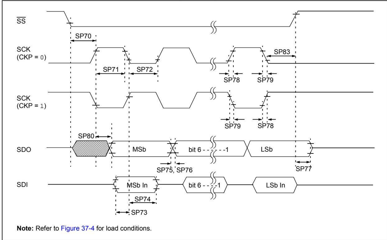
**FIGURE 37-19: SPI SLAVE MODE TIMING (CKE = 1)**
