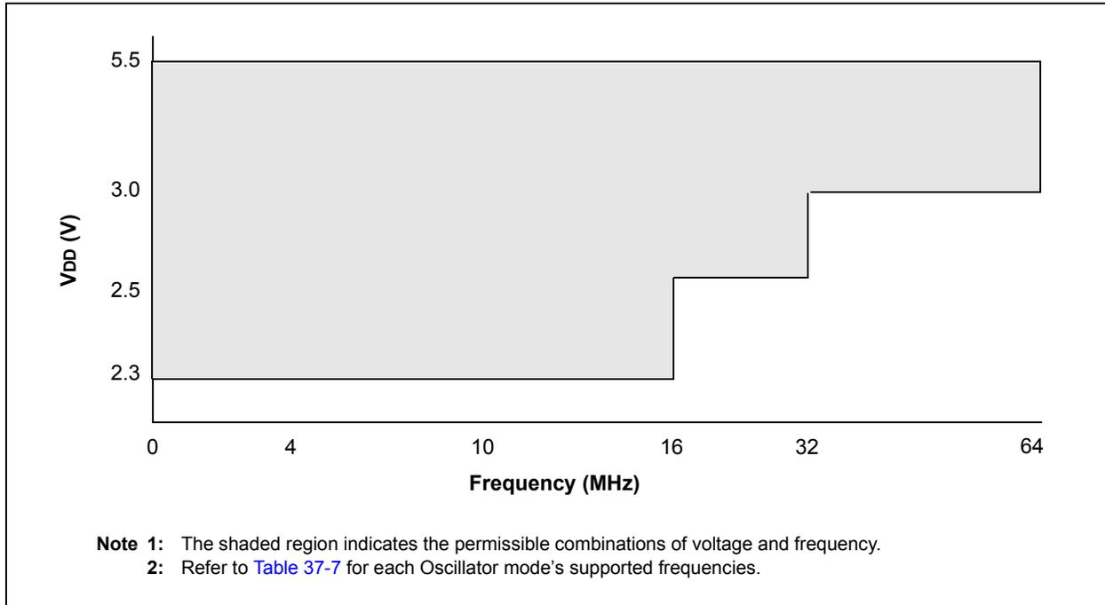
**FIGURE 37-2: VOLTAGE FREQUENCY GRAPH,  $-40^{\circ}\text{C} \leq T_A \leq +125^{\circ}\text{C}$ , PIC18LF24/25K40 ONLY**
