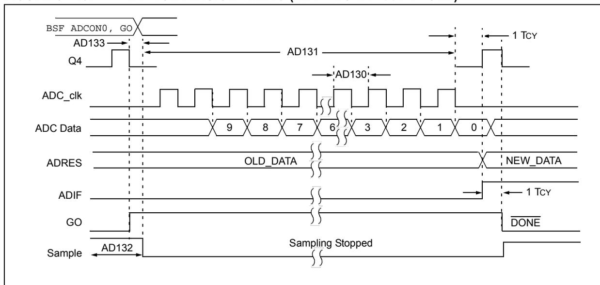
**FIGURE 37-11: ADC CONVERSION TIMING (ADC CLOCK FROM ADCRC)**
