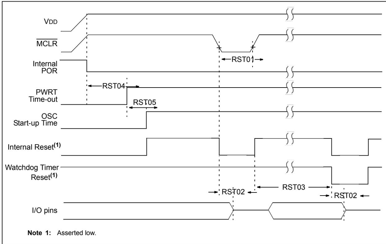
**FIGURE 37-9: BROWN-OUT RESET TIMING AND CHARACTERISTICS**
