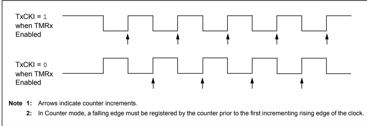
**FIGURE 19-4: TIMER1/3/5 GATE ENABLE MODE**
