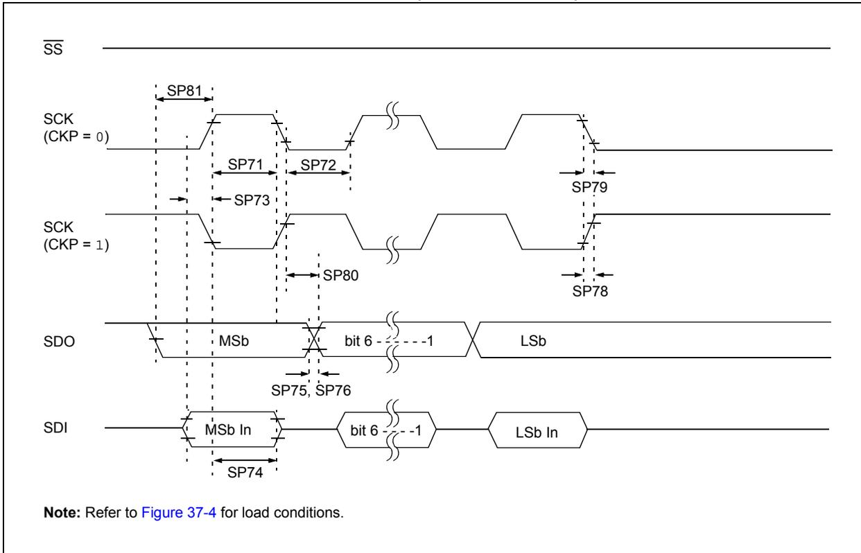
**FIGURE 37-18: SPI SLAVE MODE TIMING (CKE = 0)**
