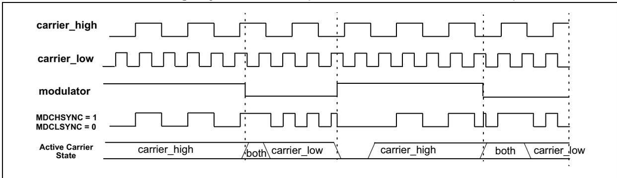
**FIGURE 25-5: Carrier Low Synchronization (MDSHSYNC = 0, MDCLSYNC = 1)**
