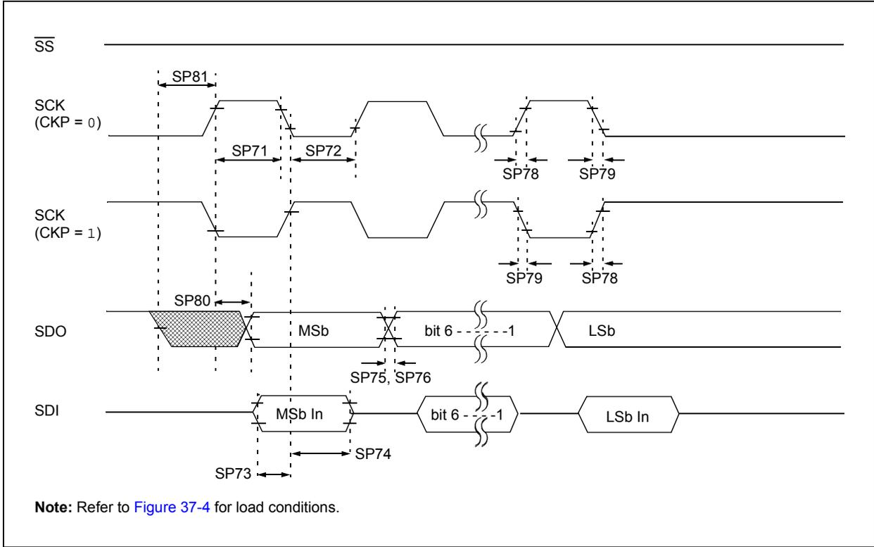
**FIGURE 37-17: SPI MASTER MODE TIMING (CKE = 1, SMP = 1)**
