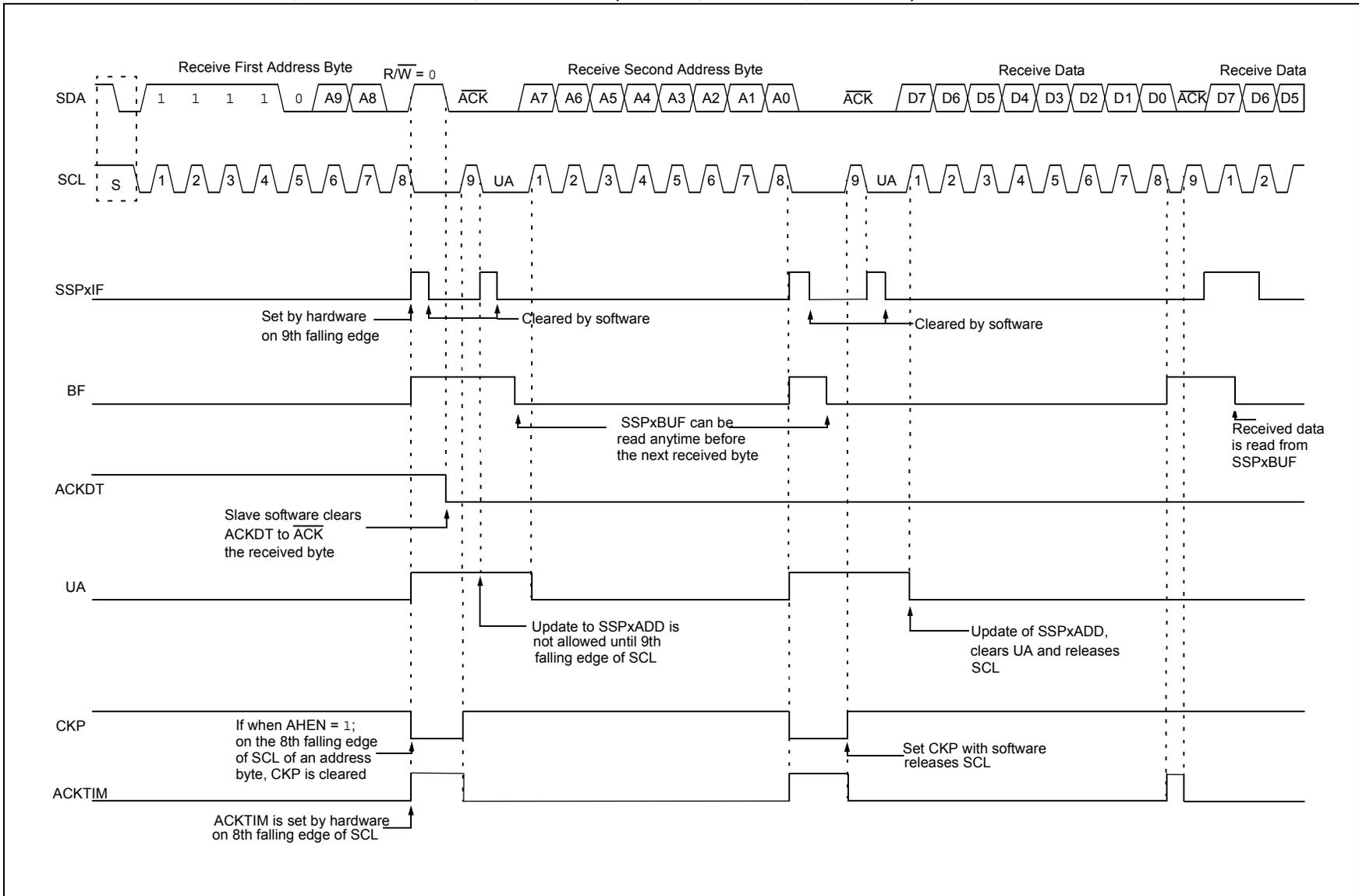
**FIGURE 26-22: I<sup>2</sup>C SLAVE, 10-BIT ADDRESS, TRANSMISSION (SEN = 0, AHEN = 0, DHEN = 0)**
