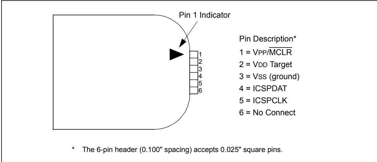
**FIGURE 34-3: TYPICAL CONNECTION FOR ICSP™ PROGRAMMING**
