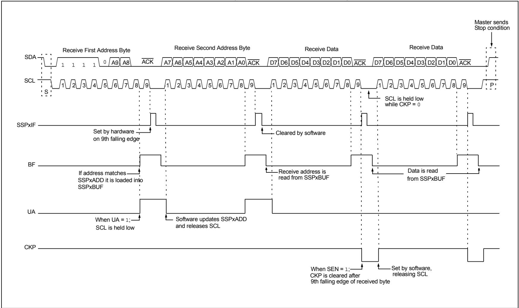
**FIGURE 26-21: I<sup>2</sup>C SLAVE, 10-BIT ADDRESS, RECEPTION (SEN = 0, AHEN = 1, DHEN = 0)**
