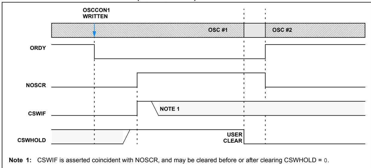
**FIGURE 4-8: CLOCK SWITCH ABANDONED**
