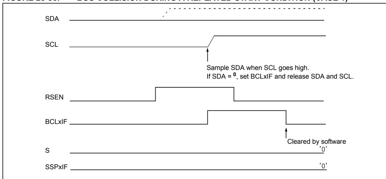
**FIGURE 26-37: BUS COLLISION DURING REPEATED START CONDITION (CASE 2)**
