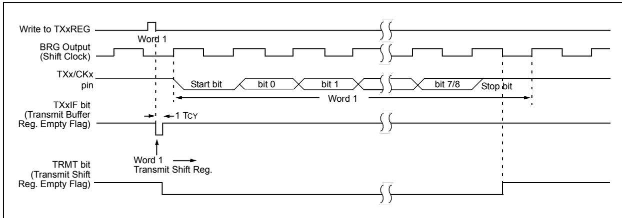
**FIGURE 27-4: ASYNCHRONOUS TRANSMISSION (BACK-TO-BACK)**
