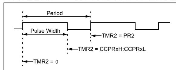
**FIGURE 21-4: SIMPLIFIED PWM BLOCK DIAGRAM**
