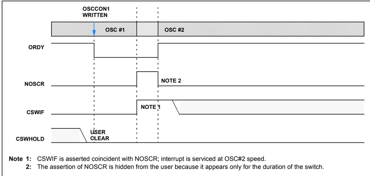
**FIGURE 4-7: CLOCK SWITCH (CSWHOLD = 1)**
