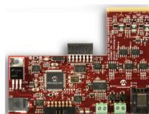
This development platform enables designers to identify and eliminate code that consumes high current, in real time. When combined with the MPLAB REAL ICE In-Circuit Emulator and MPLAB X IDE, it allows you to measure, graphically profile and optimize code power consumption for all of Microchip's PIC MCUs.
