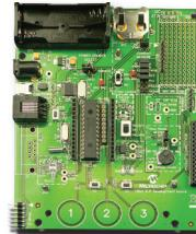
Designed with eXtreme Low Power in mind, this board enables development with the PIC24F family of 16-bit XLP PIC MCUs.
