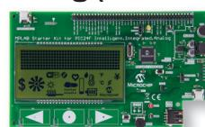
This kit features the PIC24F “GC” family with advanced integrated analog that reduces BOM cost, lowers noise and has faster throughput. Features include:
