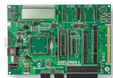
Supporting the largest number of 8-bit PIC MCUs ranging from 6 to 100 pins, the Explorer 8 Development Kit is a rapid proof-of-concept tool. Features include:
